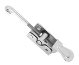
This cost effective, light duty lever operated compression hook latch provides a secure over-center action to keep panels rattle free and secure. Designed for applications where the latch and keeper are surface mounted on the same plane, folding the handle lever down pulls mating in-line panels tight.
